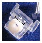
Adding to the capabilities of micro-molding is the ability to mold two different materials on the same part at the same time. The two different the rmoplastic resins are shot in sync so that it
